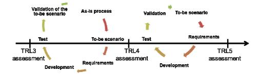
**Fig. 3.** Description of the two interlocked processes: TRL linear process and cycle usage scenario process
