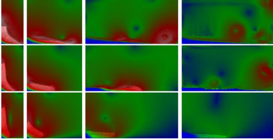
**Figure 1.** Snapshots at identical instants of the collapse of a granular column in three different fluids: air (top), water (middle), and viscous (bottom). Colors indicate the particle and fluid velocities, on the same scale (blue is slowest, white fastest).
