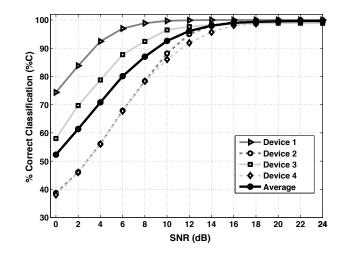
Figure 5. MDA/ML device classification performance.
