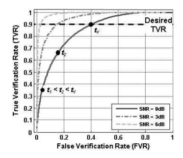
Figure 4. Device ID verification ROC curves.
