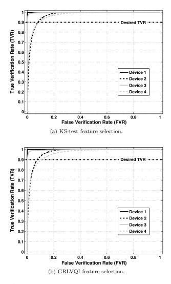
Figure 8. Authorized device ID verification for  $N_D = 4$  authorized devices.
