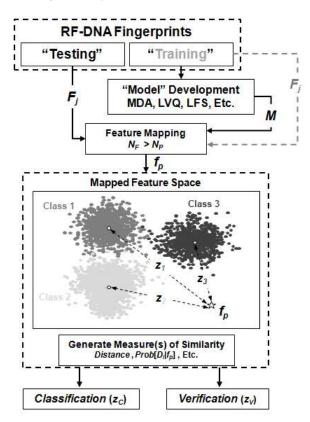
Figure 2. Block diagram of device discrimination.
