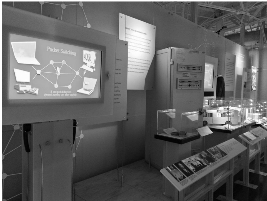
Fig. 13: A portion of the “Networking” gallery in “Revolution.” An animated video explaining packet switching is in the foreground. A refrigerator-sized IMP (Interface Message Processor) from the ARPANET, which led to the Internet, is behind.
