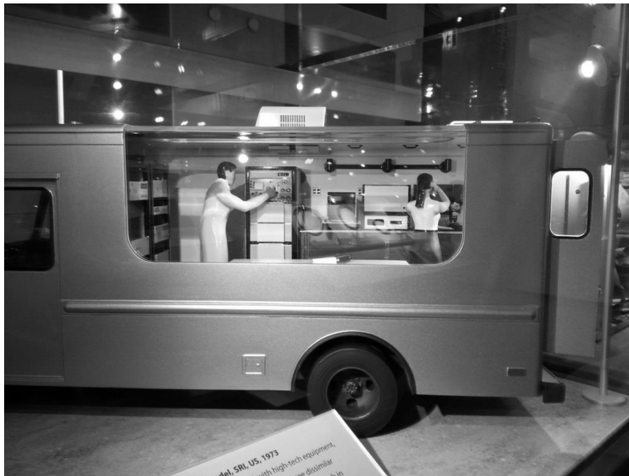
Fig. 15: Scale model of the SRI packet radio van, where the Internet, mobile data networks, and voice over IP (think Skype) were prototyped.
