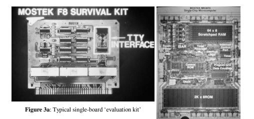
**Figure 3b**: Single-chip microcomputer: a new kind of component for the
