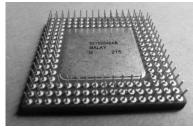
Figure 5c: Intel 80486 in 168-pin PGA (underside)
