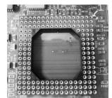
Figure 5d: Socket for PGA
