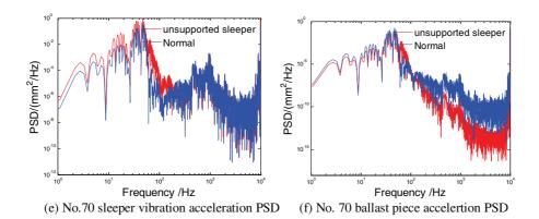
Fig. 3. Vehicle and track dynamic responses under the condition of unsupported sleeper
