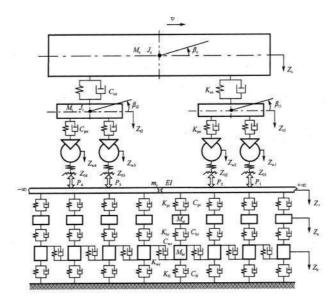
Fig. 1. Vehicle track vertical coupling model
