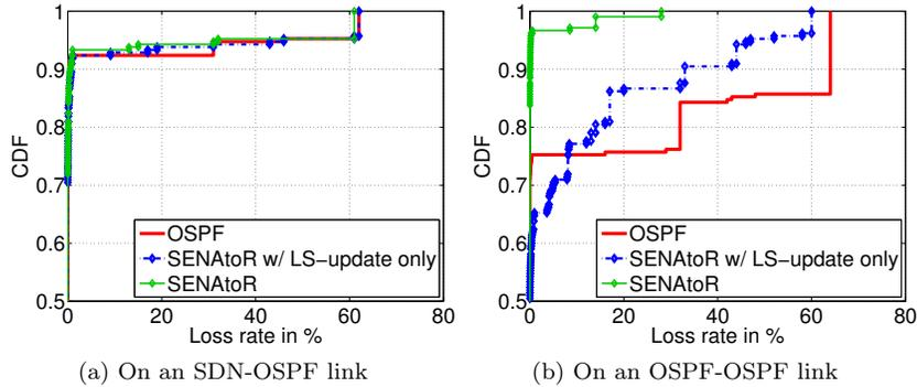
Figure 10: Link failure experiment with the atlanta topology
