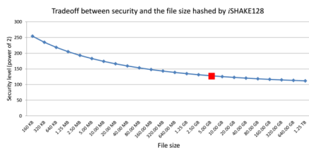
Fig. 18. A trade-off between finding collisions with the Wagner’s generalized birthday attack and the size of the hashed file with iSHAKE128
