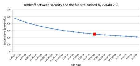
Fig. 19. A trade-off between finding collisions with the Wagner’s generalized birthday attack and the size of the hashed file with iSHAKE256
