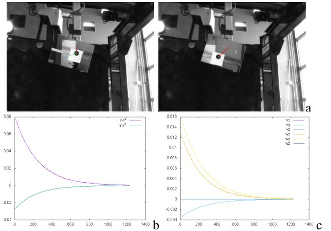
Fig. 7. Servo on one point: (a) initial position (left) and desired (and final) position (right). Video is available through youtube [here](#) and in the accompanying video ; (b) error  $\mathbf{x} - \mathbf{x}^*$ , (c) mirror velocity in mirror frame  $({}^m\mathbf{v}_m, {}^m\boldsymbol{\omega}_m)^T$  in m/s and rad/s. Note that  $(v_x, v_y$  and  $\omega_z$  are always equal to 0 as expected
