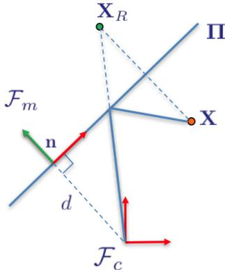
Fig. 1. Reflection and projection with a planar mirror
