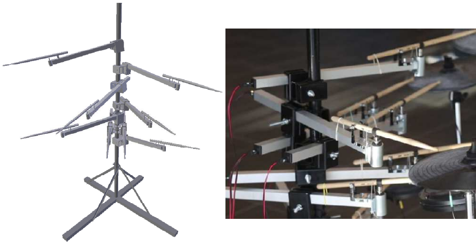
Fig. 1 Construction of the autoPRK robot
