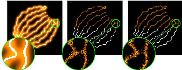
**Fig. 5.** Reconstruction results of the whole stack for the simulated dataset of Figure 4. From left to right: mean of the acquisition stack (*i.e.* wide field image) and ground truth in white, DAOSTORM reconstruction, and IRL1-CEL0 reconstruction for the best Jaccard index obtained with tolerance 250 nm. The bottom half part of the reconstructed images corresponds to the ground truth for comparison.
