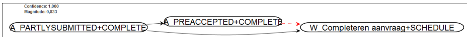
Fig. 13. Episode rules discovered in ProM for the BPIC 2012 event log. The black solid line indicates the assumed partial order (the \beta in \beta \Rightarrow \alpha ), the red dashed line indicates the added pattern (the \alpha ).
