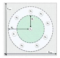
**Fig. 1.** Interference sensed by  $N_c$  due to the mobile interferers located in the annulus area  $\pi(R_o^2 - R_i^2)$ .
