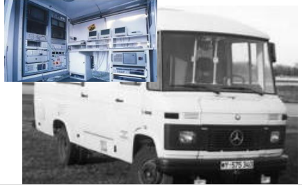
1986 VaMors (Dickmann Munich U) First autonomous vehicle on a road, Followed by EU project Prometheus
