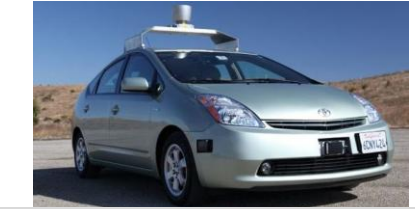
2011 Google Car project Fleet of 6 automated Toyota Prius 140 000 miles covered on California roads with occasional human interventions
