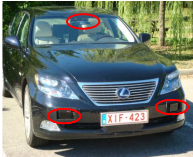
Embedded Multi-Sensors Perception => Continuous monitoring the dynamic environment
