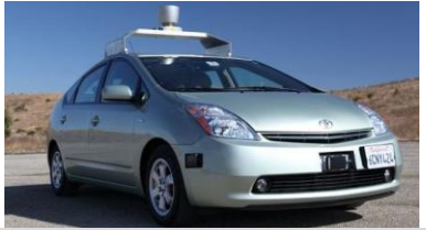
2011 Google Car project Fleet of 6 automated Toyota Prius 140 000 miles covered on California roads with occasional human interventions
