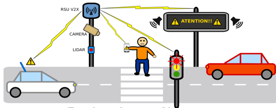
Experimental connected infrastructure
