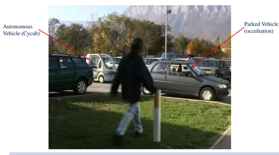
Thanks to the prediction capability of the BOF technology, the Autonomous Vehicle "anticipates" the behavior of the pedestrian and brakes (even if the pedestrian is temporarily hidden by the parked vehicle)
