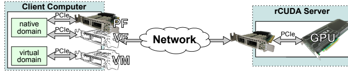
Fig. 4. Testbed used in the experiments presented in this paper. The client node, hosting the KVM VM, owns an InfiniBand ConnectX-3 network adapter, which has been virtualized. The server node also owns an InfiniBand ConnectX-3 network adapter. Notice that the tests in this paper will always use the real instance of this latter adapter, which has not been virtualized.
