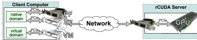
Fig. 4. Testbed used in the experiments presented in this paper. The client node, hosting the KVM VM, owns an InfiniBand ConnectX-3 network adapter, which has been virtualized. The server node also owns an InfiniBand ConnectX-3 network adapter. Notice that the tests in this paper will always use the real instance of this latter adapter, which has not been virtualized.
