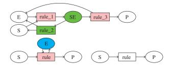
**Fig. 1.** Reaction graphs of the Michaelis–Menten enzymatic reaction, either complete with intermediary complex SE, or reduced with or without enzyme E. The first reduction can be achieved with the graphical operations explained in Section 2.2, for example by merging the reaction nodes  $rule\_1$  and  $rule\_3$  in pink into a reaction node rule and by deleting the green nodes SE and  $rule\_2$ . The second reduction simply deletes the blue node E.
