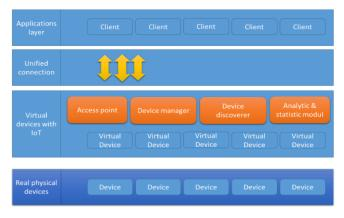
Fig. 3. Concept definition of IoT in the industry.
