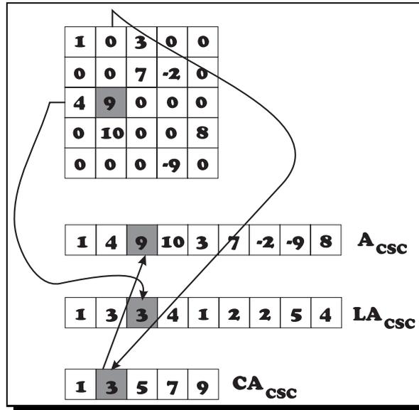
FIG. 3.3 – *Format CSC (Compressed Sparse Column)*
