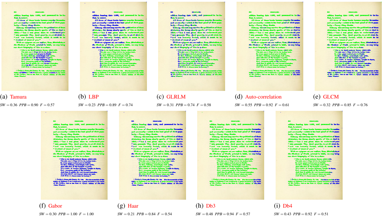
Fig. 11: Examples of resulting images of the proposed pixel-labeling scheme for comparing the nine investigated texture-based feature sets on the “Only two fonts” category of HDIs from the HBR2013 dataset.
