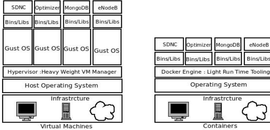
Fig. 2: (a) Virtual machine vs. (b) Docker container architecture
