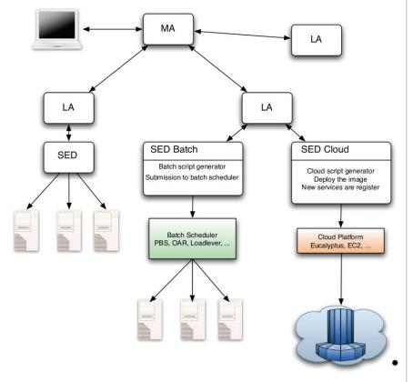
Figure 1: The cloud-enabled DIET hierarchy.
