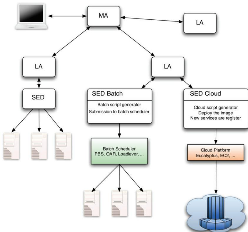
Figure 1: The cloud-enabled DIET hierarchy.
