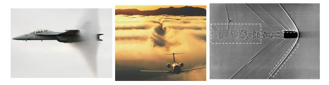
Figure 2: Left, shock waves (Mach cone) emitted by a supersonic F-14 fighter. Middle, turbulent wake of a transsonic Falcon business jet. Right, schlieren picture showing the flow pattern around a bullet at supersonic speed. Dotted white squares exhibit different components of the flow features: boundary layer near body, shock waves in the far-field and turbulent flow in the wake.
