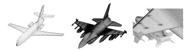
Figure 1: Left, surface mesh of a falcon business jet geometry dating back to the early 90's; it is composed of 1,879 vertices. Middle, surface mesh of a F-16 fighter geometry mid 2000. It is composed of 271,763 vertices. Right, close view of the F-16 surface mesh. Note the high accuracy of the details on the geometry.
