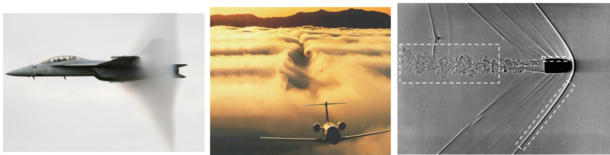
Figure 2: Left, shock waves (Mach cone) emitted by a supersonic F-14 fighter. Middle, turbulent wake of a transonic Falcon business jet. Right, schlieren picture showing the flow pattern around a bullet at supersonic speed. Dotted white squares exhibit different components of the flow features: boundary layer near body, shock waves in the far-field and turbulent flow in the wake.
