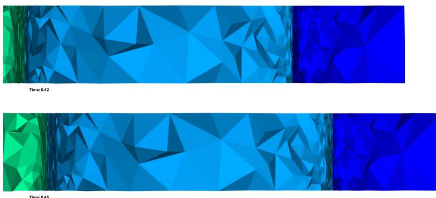
Figure 10: Zoom on the mesh and solution at the beginning (top) - t = 0.42 - and at the end (bottom) - t = 0.45 - of the fourteenth sub-interval. One can see the two waves move forward inside the adapted bands while the refined bands are moving forward.
