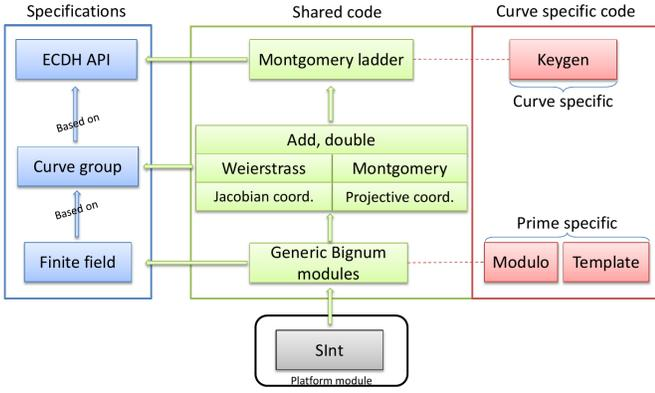
Fig. 2. Architecture of our verified elliptic curve library
