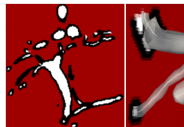
Fig. 8 (Left) The porosity map of Fig 1 created from the vessels segmentation. The porosity is 1 in the vessels (in white), 0.04 in the endothelium (in black) and 0.1 in the parenchyma. (Right) Zoom on the porosity map. The extremities of the vessels are detected using the centerlines so that the blood flow can go through the vessel.
