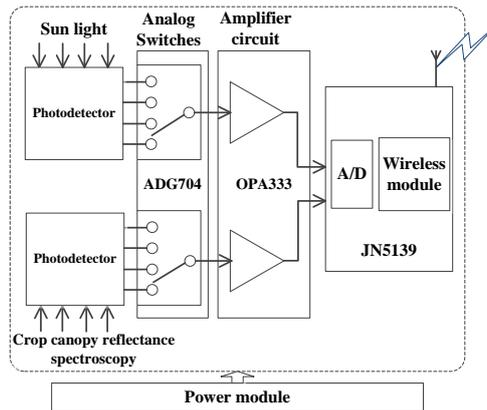
Fig. 2. Block diagram of intelligent sensor node
