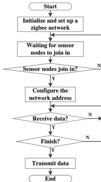
Fig.5 Flow chart of the software in coordinator
