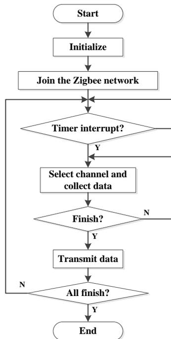
Fig. 3. Flow chart of software in sensor node
