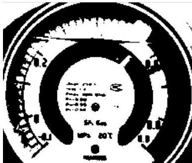
Fig. 6. Automatic threshold segmentation
