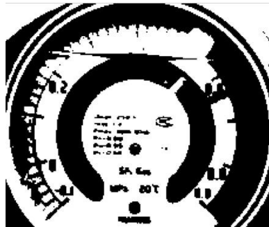
Fig. 6. Automatic threshold segmentation
