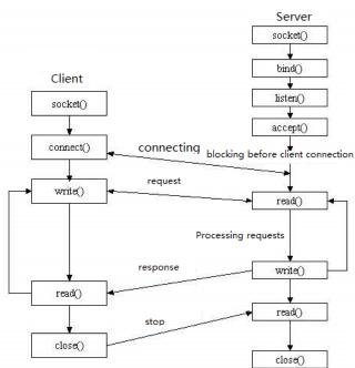
Fig. 2. Working procedure of Socket
