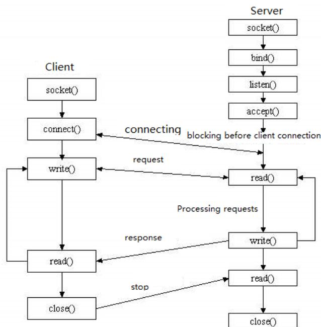
Fig. 2. Working procedure of Socket
