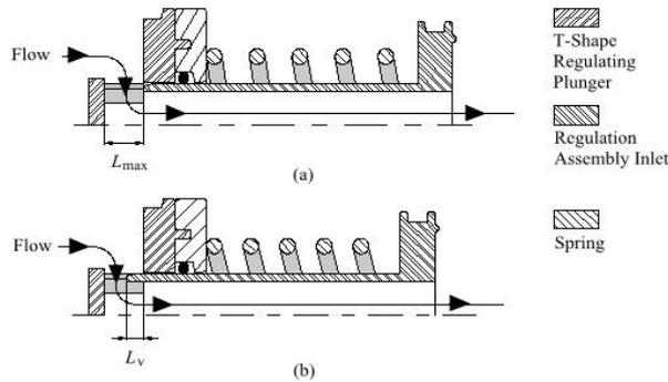
Fig. 2. Regulating process of a pressure regulation assembly (the axisymmetric part)
