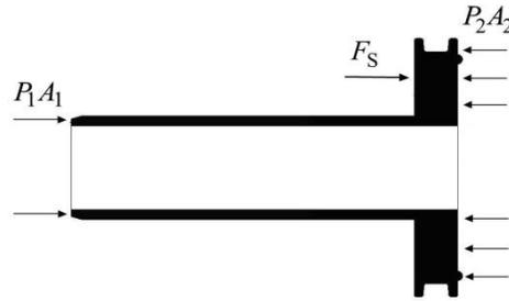
**Fig.3.** Force acting on the T-shape regulating plunger
