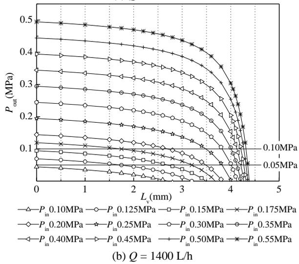
**Fig. 7.** Outlet pressure change with different displacements at different inlet pressures ( $L_{\max} = 5 \text{ mm}$ )
