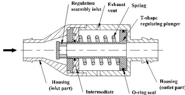
Fig. 1. Schematic cross-section of a pressure regulator
