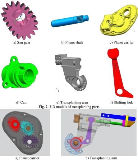
Fig. 3. Sub assembly of transplanting mechanism
