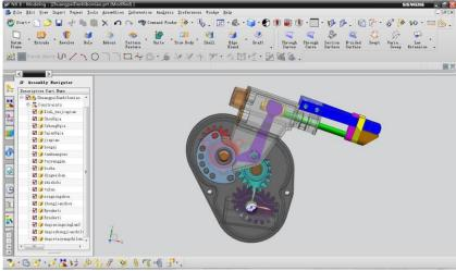
Fig. 4. 3-D virtual prototype model of transplanting mechanism
