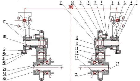
Fig. 6. 2-D assembly drawing of transplanting mechanism
