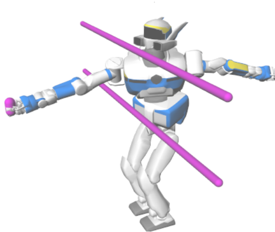
Fig. 1 As a typical example, proposed in [2], a humanoid robot is assigned with the following objectives: 1. Maintain balance; 2. Avoid collisions; 3. Reach an object; 4. Keep this object within sight.
