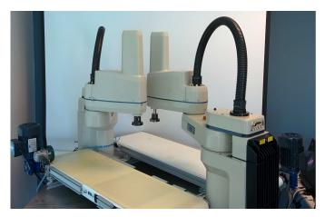
Fig. 1: Experimental setup. Two Adept Cobra SCARA [3] robots sharing the same working environment.
