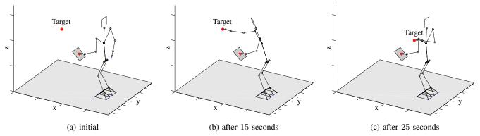
Fig. 1: Test 2: configurations of the robot during the simulation. Grey areas represent contact surfaces.
