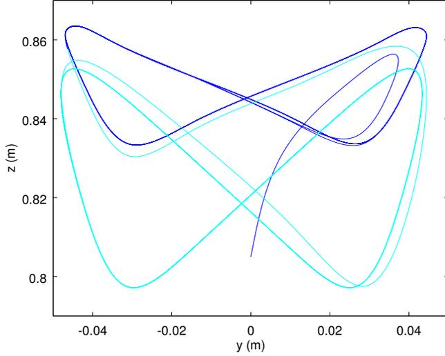
Fig. 4. Trajectory of the CoM of the robot in the frontal plane when walking on a flat, even ground, starting from rest and reaching a speed of  $0.2 \text{ m.s}^{-1}$  (dark blue), then transitioning to a speed of  $0.6 \text{ m.s}^{-1}$  (light blue). The typical butterfly shape and how it changes with walking speed matches what is measured in human walking [34].
