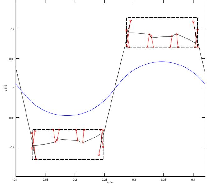
Fig. 5. Trajectories of the CoP (black curve) and CoM of the robot (blue curve), footprints (dashed rectangles), and bounds introduced in Section II (red segments), shown here every  $100 \text{ ms}$ . We can check that the CoP always stays within these bounds, and that these bounds always stay within the footprints, as desired, guaranteeing the dynamic feasibility of the generated 3D walking motion.
