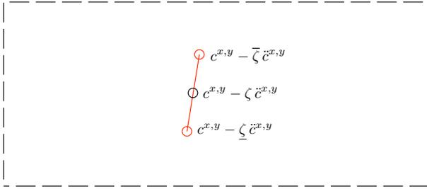
Fig. 1. If we make sure that  $c^{x,y} - \zeta \ddot{c}^{x,y}$  and  $c^{x,y} - \bar{\zeta} \ddot{c}^{x,y}$  are in the convex hull of the contact points (here the dashed rectangle), then we know that the CoP  $c^{x,y} - \zeta \ddot{c}^{x,y}$ , which lies somewhere in-between, also lies in this convex hull, and dynamic feasibility is guaranteed.
