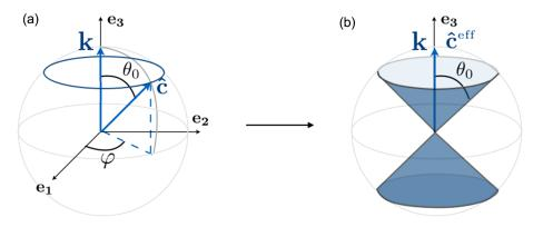
**Figure 2.** First configuration of a VTI girdle with a single zenith angle  $\theta_0$ . (a) shows a typical c axis  $\hat{c} = (\sin \theta_0 \cos \varphi, \sin \theta_0 \sin \varphi, \cos \theta_0)$  within one grain, with a constant  $\theta_0$ , and  $\varphi$  varies randomly from grain to grain. (b) shows the resulting VTI texture of the polycrystal at the macroscopic scale.  $\hat{c}^{\text{eff}}$  is the effective c axis.
