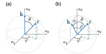
**Figure 5.** (a) System of angles used in Bennett's calculations.  $\hat{c}$  is given by  $(\varphi, \theta)$  and k is given by  $\sigma$ , being otherwise in the  $(e_1, e_3)$  plane. The extra angle  $\hat{\theta}$  denotes the angle between k and  $\hat{c}$ , thus  $\cos\hat{\theta} = \sin\sigma \cos\varphi \sin\theta + \cos\sigma \cos\theta$ . (b) Particular case of the Bennett configuration, for  $\sigma = 0$ ; in this case,  $\hat{\theta} = \theta$ .
