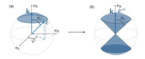
Figure 3. Second configuration of the usual VTI clustered texture. (a) shows a typical  $c \, axis \, \hat{c} = (\sin\theta \, \cos\varphi, \, \sin\theta \, \sin\varphi, \, \cos\theta)$  within one grain, where  $\theta$  varies in  $[0, \theta_0]$  and  $\varphi$  varies randomly from grain to grain. (b) shows the resulting clustered, VTI, texture of the polycrystal at the macroscopic scale.  $\hat{c}^{\text{eff}}$  is the effective c axis.
