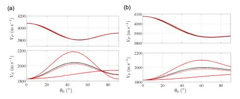
**Figure 4.** Illustration of the inconsistency of the velocity averaging method for the two VTI textures shown in Fig. 2a and b. The velocities  $V_P$  and  $V_S$  are reported as functions of  $\theta_0$ , from the effective medium theory (black curves) and from the velocity averaging method (plain red lines). The dotted red lines show the shear wave velocity from Bennett's expression, close to the harmonic mean of the two unphysical shear wave velocities in plain red line.
