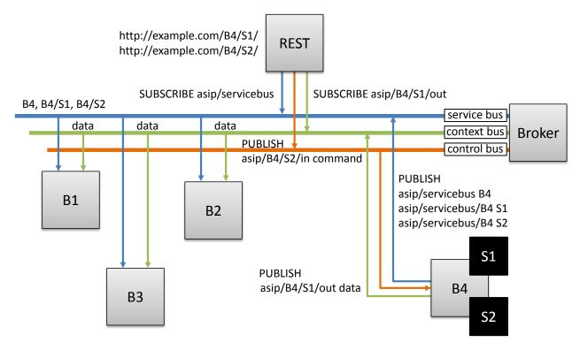
Figure 3: An application scenario exploiting the service discovery functionality.
