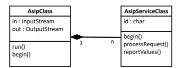
Figure 1: ASIP simplified class diagram
