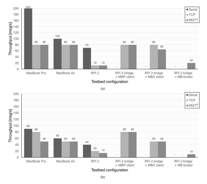
Figure 6: Throughput for Java (a) and Python (b) clients with various testbed network configurations.
