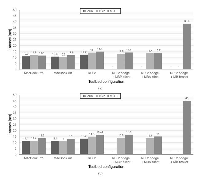
Figure 8: Latency for Java (a) and Python (b) clients with various testbed network configurations.
