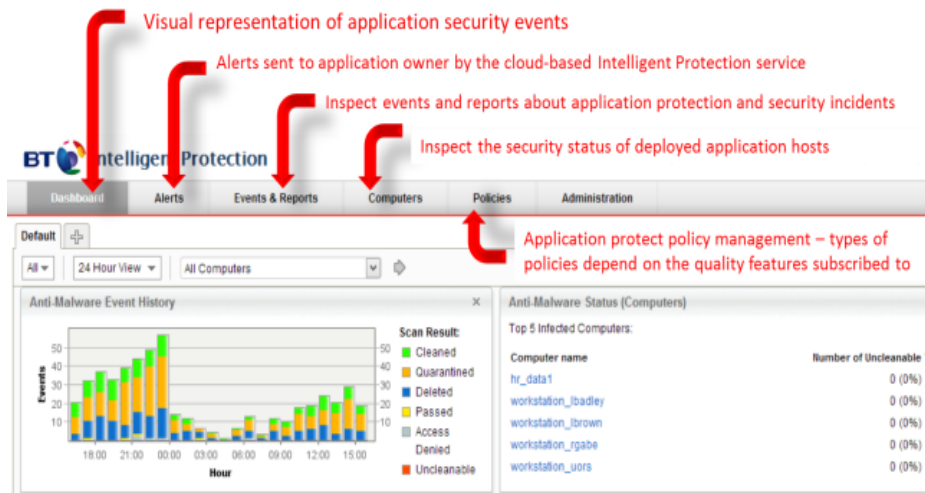
Fig. 4. Example of Intelligent Protection Dashboard
