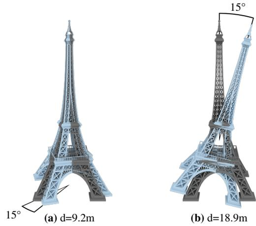
**Fig. 3** Usual metrics would consider the distances between the two poses in cases (a) and in (b) equal – as in both cases the two poses are linked by a rotation of  $15^\circ$  around the center of mass of the object. Our distance accounts for the object geometry and discriminates these two configurations.
