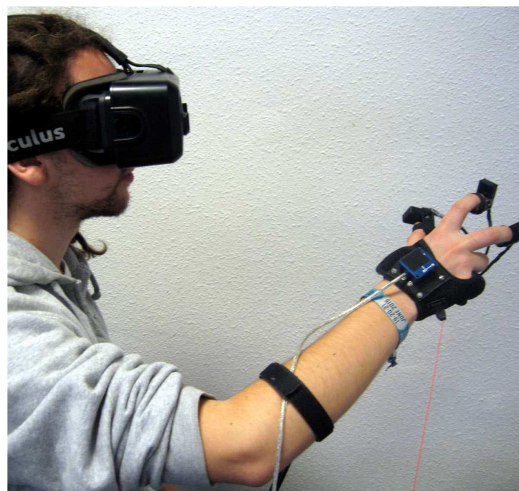
FIGURE 7 | Immersive VR setup used to test the proposed tactile rendering techniques.
