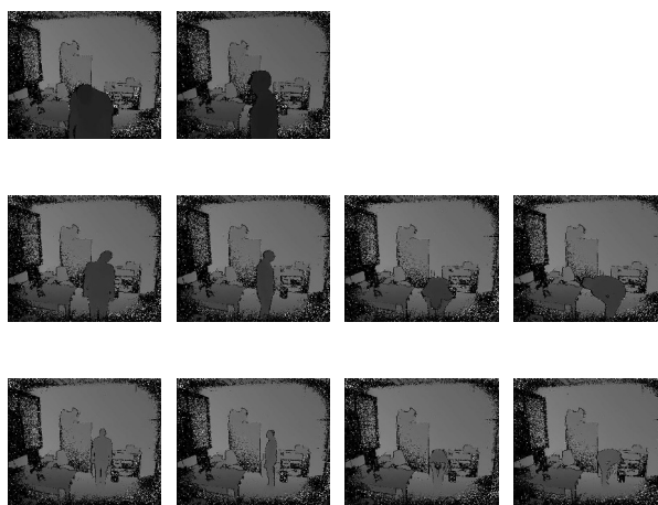
Figure 1. Examples of depth maps of standing (the first two columns) and bending (the 3rd and 4th columns) postures in full 360° views to a Kinect2 sensor and with different head poses. Depth maps of the three rows correspond to the distance of one, two and three meters to the Kinect2 sensor.
