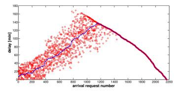
Fig. 7. Random realization of queuing delays of the activation requests arrived during the control interval for constant D values (blue) and uniform D values in [60min, 120min] (red), U = 3000, K = 400KW.
