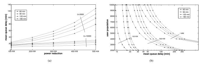
Fig. 6. Design curves with mean service delays vs. power reduction (a) and user population vs. mean service delays (b) under different control periods.
