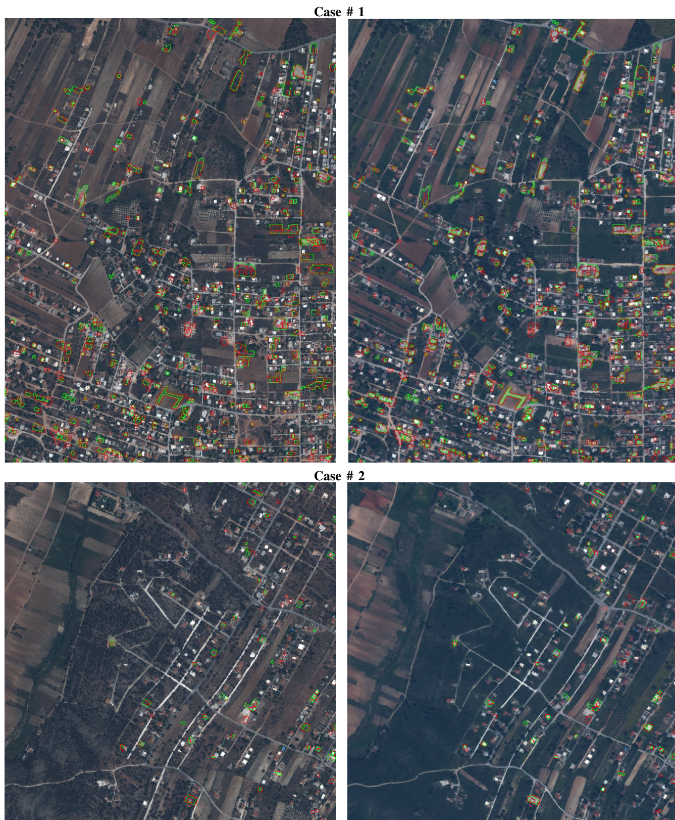
Fig. 6: Experimental results after the application of the developed change detection framework based on the unsupervised formulation ( E_{ch} from equation (6)) for two sub-regions (case #1 and case #2) of the study area. The detected changes are shown with red color and the ground truth data with green. Both are superimposed onto the very high resolution satellite images acquired in 2006 (Quickbird, left) and 2011 (Worldview-2, right).
