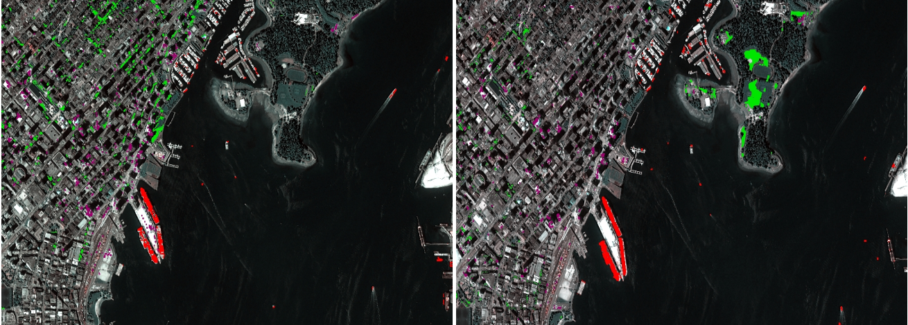
Fig. 4: Change Detection from multitemporal, multi-sensor between: (a) a Deimos March'15 and a Deimos May'15 ( D1-D2 , left), (b) an Iris video sequence (first frame) and a Deimos May'15 ( V-D2 , right).
