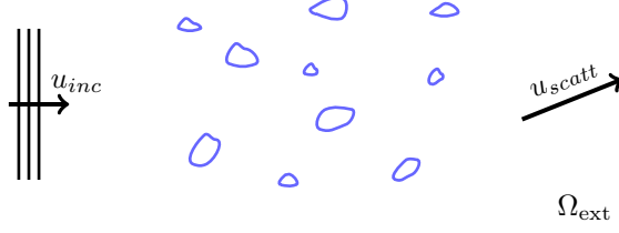
Figure 1: Scattering of a planewave by various and non-overlapping obstacles.
